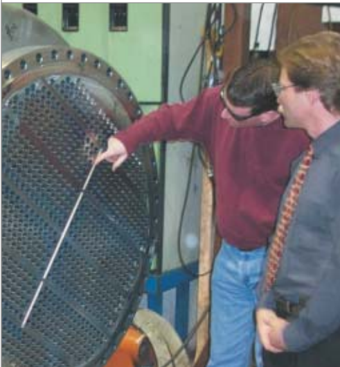
Ellett's David Clift (right) says that "everything had to be perfect" in fabricating the atypical heat exchanger. The tube holes [pointed out by Jim Hunt (left)] were drilled to tight tolerances.
